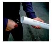
The inside of the pipe needs to be perfectly smooth (use a file and if necessary a scouring pad) to ensure there is no residual PVC inside the pipe for fluff to catch on.
