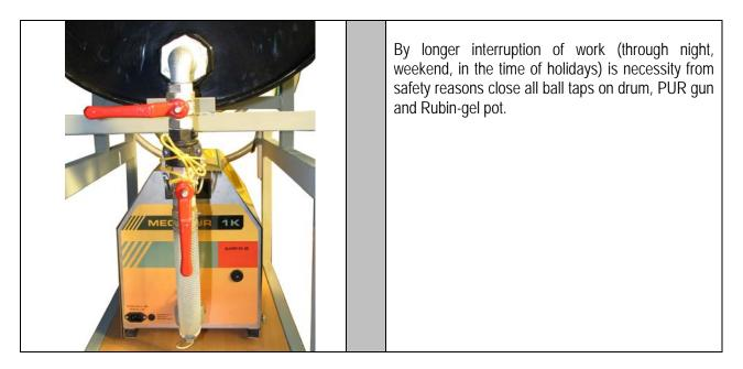
By longer interruption of work you need weekly to let off through system 250 g of glue in proper close can. This procedure assure faultless functionalism of the system.
